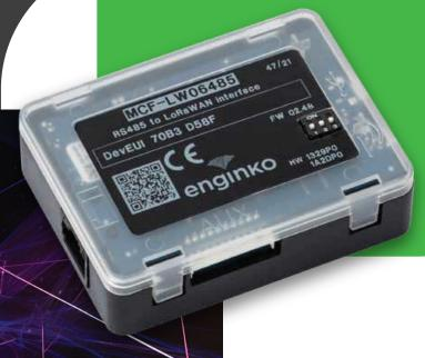
This interface can be connected to any Modbus device to read and write any register of the connected device through the LoRaWAN® platform. Configuration is simply made using a configuration file uploaded to the interface via USB or downlink.
